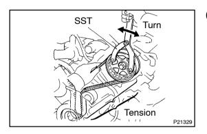
(c) Using SST, turn the LH camshaft timing pulley counterclockwise until there is tension between the crankshaft timing pulley and LH camshaft timing pulley.
