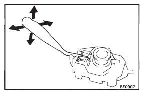
(c) After installing the light control switch to the switch body, insure that the switch operation is smooth.
