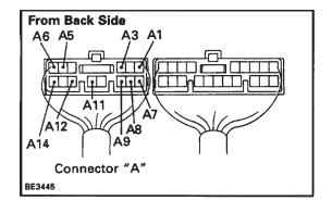
(c) Connect the wire harness side connector to the combination switch and inspect wire harness side connector from the back side as shown.
