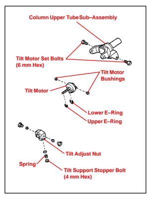
increments until snug. Torque the Tilt Motor Set Bolts to 20 N•m (210 kgf•cm, 15 ft•lbf).
