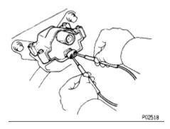
3. Using an ohmmeter, measure the resistance between the positive (+) and negative (-) terminals. **Primary Coil resistance (Cold): 0.36 - 0.55 Ohms Primary Coil resistance (Hot): 0.45 - 0.65 Ohms** If the resistance is not as specified, replace the Ignition Coil.
