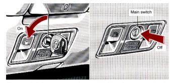
The trunk lid opener can be used when the master key is inserted into the main switch under the dash panel and turned counterclockwise. When the main switch is pushed in, the trunk lid opener cannot be used. The opener is turned off by pushing the main switch in.
