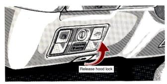
To open the hood, pull the hood lock release lever under the dash. The hood will spring up slightly.
