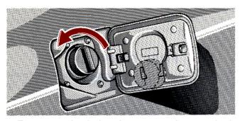
2. To remove the fuel tank cap, turn the cap slowly counterclockwise, then pause slightly before removing it. The removed cap can be stored on the back side of the fuel filler door.
