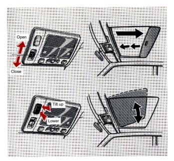
To slide open or to close the moon roof, push the switch to the OPEN or CLOSE side. To tilt up or lower the rear end of the moon roof, push the switch on the TILT UP or DOWN side.
