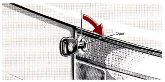
To open the trunk lid, insert the master key and turn it clockwise.
