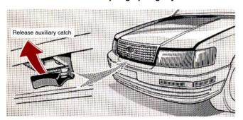
In front of the vehicle, pull the auxiliary catch lever and lift the hood.
