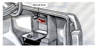
Pull the manual lever at the back right of the trunk.
