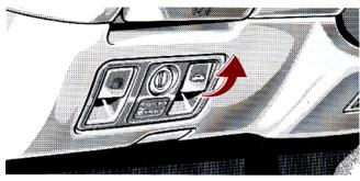
To open the trunk lid while sitting in the driver's seat, pull the lever with the main switch on.
