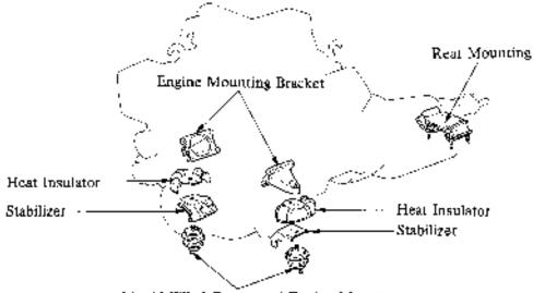
Liquid-Filled Compound Engine Mounts
