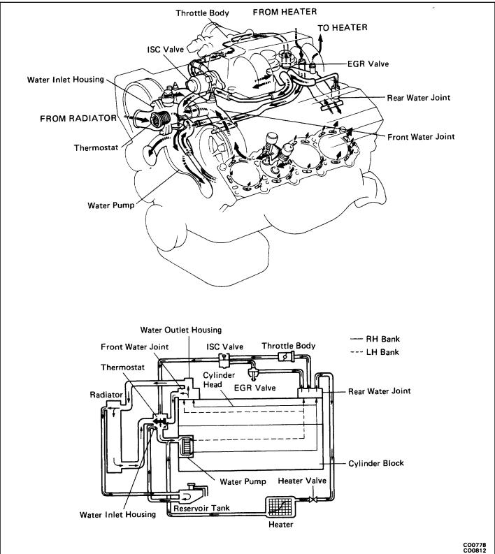
Coolant which is heated in the water jacket is pumped to the radiator, through which a cooling fan blows air to cool the coolant as it passes through. Coolant which has been cooled is then sent back to the engine by the water pump, where it cools the engine.
