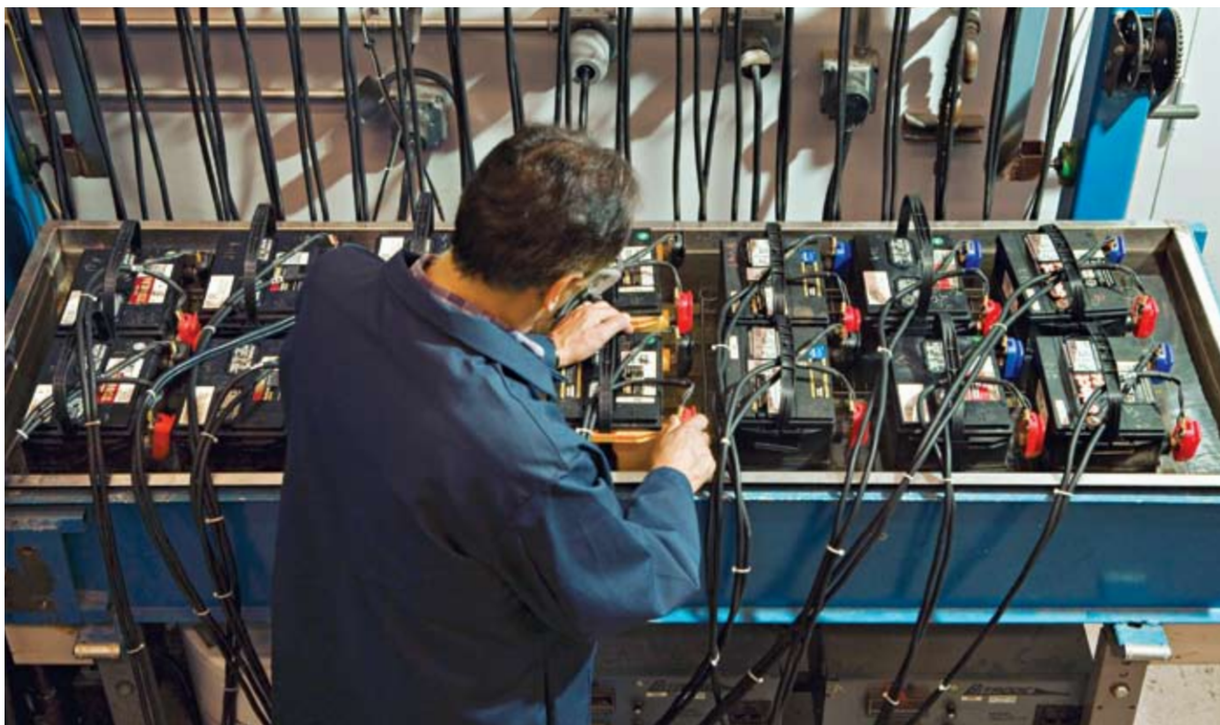
POWER DRAIN Technician Vincent Leonardis measures how each battery holds up after being drained and recharged almost 3,000 times.
