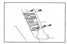
REMOVE RADIO WITH A/C CONTROL ASSEMBLY Remove four screws and radio with the A/C control assembly.
