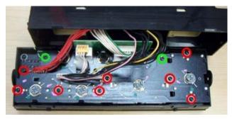
1. After the LCD climate unit is separated, there are two side screws that need to be removed.
