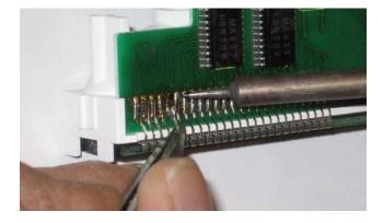
6. Set aside the face. Then carefully turn the PCB-LCD module so that solder side of the LCD is up and accessible to be removed with the soldering iron.
