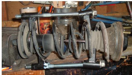
Remove shaft retaining nut and upper mount.
