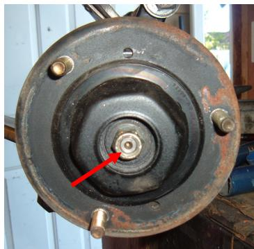
Carefully remove spring from strut. Place new strut assembly securely in vise and install spring and upper mount. Make sure that bottom of spring is seated correctly (there is an obvious indent in the bottom support to accept the end of the spring.)
