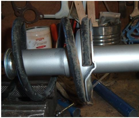
Make sure that the top of the spring is aligned with the mark on the upper mount. Release the spring compression tool.
