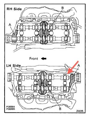
NOTICE: Do not drop the adjusting shim into portions A and B. If dropped into portion A, the adjusting shim will pass through the cylinder head and cylinder block into the oil pan. If dropped into portion B, the adjusting shim cannot be recovered without removing the exhaust camshaft.
