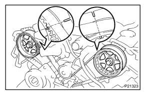
(c) Check that each pulley aligns with the timing marks as shown in the illustration.
