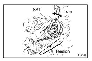
(c) Using SST, turn the LH camshaft timing pulley counterclockwise until there is tension between the crankshaft timing pulley and LH camshaft timing pulley.
