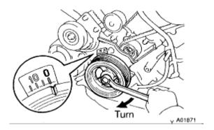
a. Turn the crankshaft pulley and align its groove with timing mark "0" of the No.1 timing belt cover.
