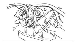
TIMING BELT GUIDE Install the belt guide, facing the cup side outward.
