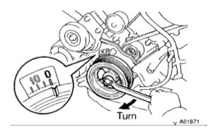
b. Slowly turn the crankshaft pulley **2 revolutions** from TDC to TDC. **NOTICE:** Always turn the crankshaft pulley clockwise.
