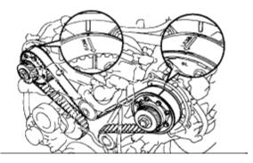
b. Check that the timing marks of the camshaft timing pulleys and timing belt rear plates aligned. If not, turn the crankshaft **1 revolution**  $(360^{\circ})$ .
