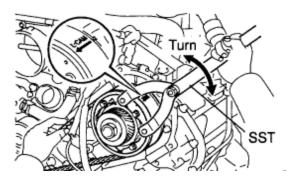
b. Using SST, turn the timing pulley. Align the installation mark on the timing belt with the timing mark of the timing pulley, and hang the timing belt on the timing pulley. SST 09960-10010 (09962-01000, 09963-00350)
