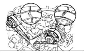
c. Check that each pulley aligns with the timing marks as shown in the illustration. If the timing marks do not align, remove the timing belt and reinstall it.
