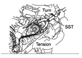
c. Using SST, turn the LH camshaft timing pulley counterclockwise until there is tension between the crankshaft timing pulley and LH camshaft timing pulley. SST 09960-10010 (09962-01000, 09963-00350)
