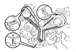
IF RE-USING TIMING BELT, CHECK INSTALLATION MARKS ON TIMING BELT Check that there are 3 installation marks on the timing belt by turning the crankshaft pulley as shown in the illustration.
