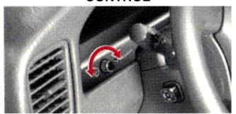
To adjust the brightness of the instrument panel lights, turn the knob.
