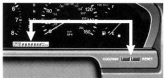
This meter displays the odometer and two trip meters. To change the mode indication, push the "ODO/TRIP" button.
