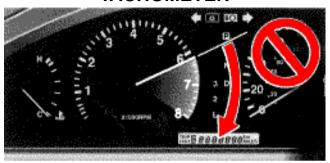
The tachometer indicates engine speed in thousands of rpm (revolutions per minute). Use it while driving to prevent engine overrevving.
