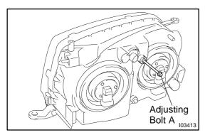
(i) When the paper is not lighted up properly, using the adjusting bolt A, adjust the lights in the vertical direction.
