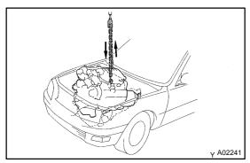
(f) Lift the engine out of the vehicle slowly and carefully. HINT:
