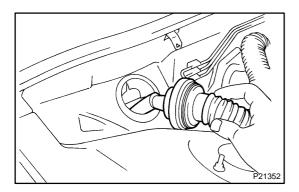
(f) Disconnect the grommet from the cowl panel, and pull out the engine wire.
