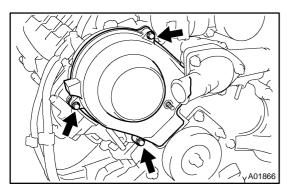
8. REMOVE DRIVE BELT, FAN, FLUID COUPLING AND FAN PULLEY
