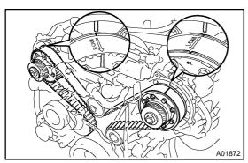
(c) Check that each pulley aligns with the timing marks as shown in the illustration.
