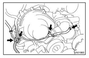
(d) Install the radiator reservoir outlet pipe to the RH cylinder head and timing belt cover with the bolt and nut.
