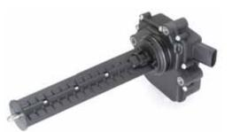
The intake manifold tuning valve separates the intake plenum into halves, with each bank of the engine breathing through its own half at lower revs for improved torque, but opening to provide access to the entire intake manifold volume at higher rpm for maximum top-end power.
