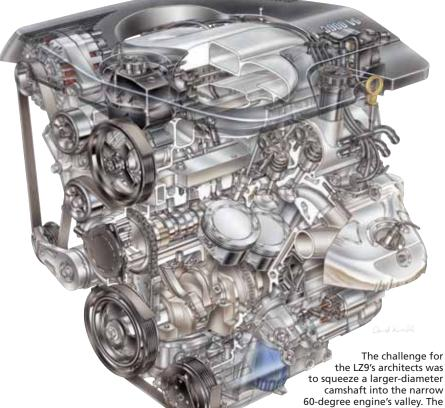
camshaft into the narrow 60-degree engine's valley. The solution was to push the cylinders down 1.5 mm (0.06 in) from the top of the block, widening the area where the cam resides.
