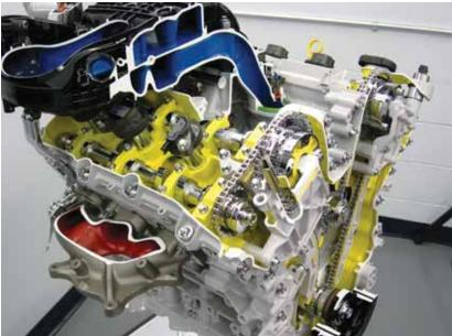
Cam phasers on intake cams deliver high-value emissions performance on the newest V6 engine from Ford.
