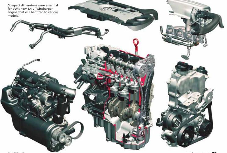
The sum of its parts: VW's new turbocharged and supercharged four-cylinder engine.
