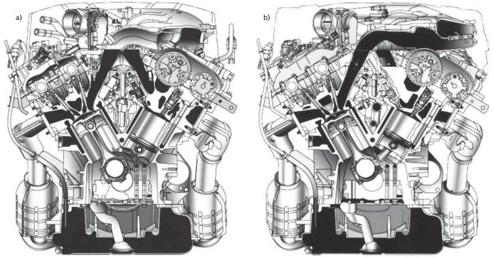
The cross sections show: a) the D-4S engine with direct and port injectors, and b) the 3GR-FSE direct-injection D-4 version.
