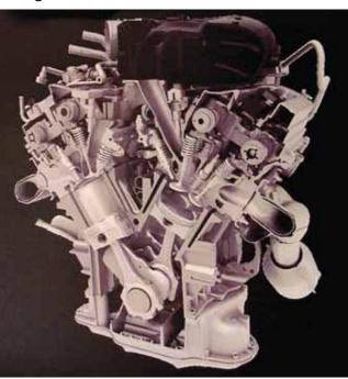
The 2GR-FSE engine for Lexus applications initially gets port and direct injectors.
