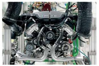
To ensure continuous quality, each of the hand-assembled M5 engines runs for 20 min on a dynamometer to confirm its correct operation, and some engines are tested randomly for two hours.
