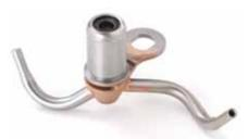
Although piston oil cooling jets were pioneered on high-performance air-cooled motorcycle engines that needed to cool the piston crowns, GM uses the jets to help quiet the engine, as the pistons slide more easily in their bores. aei tech briefs
