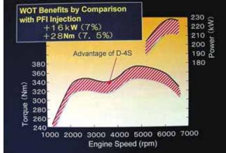
Shaded area shows improved torque by D4-S dual injection.
