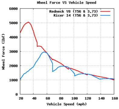
Figure 5: Plot of rear wheel force versus vehicle speed for Redneck and Ricer when using a Tremec T56 transmission and 3.73 axle ratio.
