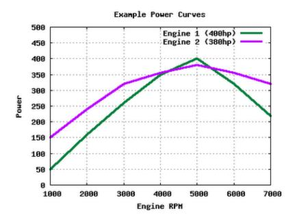
Engine 1 has more peak power than engine 2, but engine 2 has more average power across the rev range. Engine 2 would make for a faster car in most cases.
