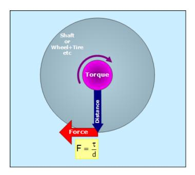
Torque can be used to create a force at a distance, as seen below. On a car, this is how the wheel and tire apply force to the pavement.
