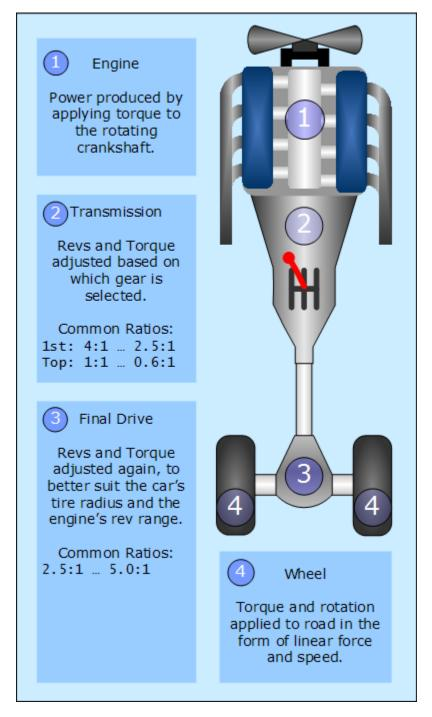
The drivetrain of a car is fitted with a transmission and final drive gearing to adjust the engine's torque and revs to accelerate the car.
