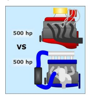
The car with the V8 will be named **Redneck**, and the car with the 4 cylinder will be named **Ricer**. The V8 can rev to 6000RPM and produce a ton of torque, while 4 cylinder can to rev way up to 9000RPM and produce a fair bit of torque. To keep the math very simple, the V8 idles at 600RPM, and the I4 idles at 900RPM. Below are plots of the two fictitious engine's torque and power curves.
