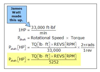
Shaft power in horsepower
