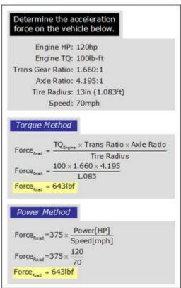
The calculated acceleration force is the same when using the torque method or the power method.
