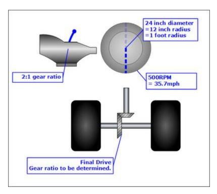
Details of the drivetrain layout.
