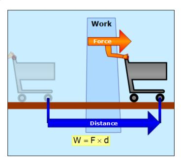
Work is done on the object by applying a force along a distance
