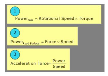
The wheels receive torque and rotational speed from the engine, and lay down a force onto the pavement. It is this force which accelerates the vehicle. The car's speed is directly related to the rotational speed of the wheel.
