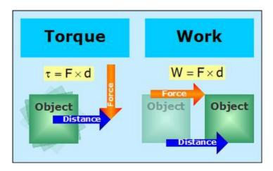
The difference between torque and work
