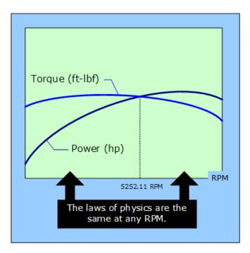
5252RPM is not a significant point in a physical sense. It is merely the RPM at which a graph of torque in pound-feet and power in horsepower would cross when drawn on the same piece of paper. If different units were used, the curves would cross at a different point, yet the principles of operation would remain unchanged.
