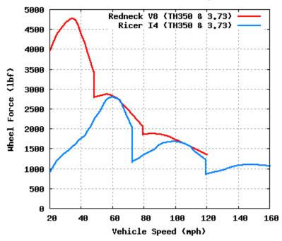
Figure 4: Plot of rear wheel force versus vehicle speed for Redneck and Ricer when using a TH350 transmission and 3.73 axle ratio. The steep vertical drops are the gear changes at redline. Gear changes take place instantaneously for simplification.
