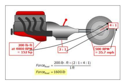
The red engine makes 152 horsepower, which is twice the power of the other two engines. It is putting a 1600 lb force to the road, which is also twice as high as the other two engines.
