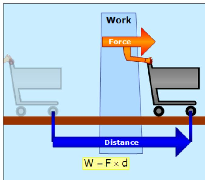
*Work is done on the object by applying a force along a distance*
