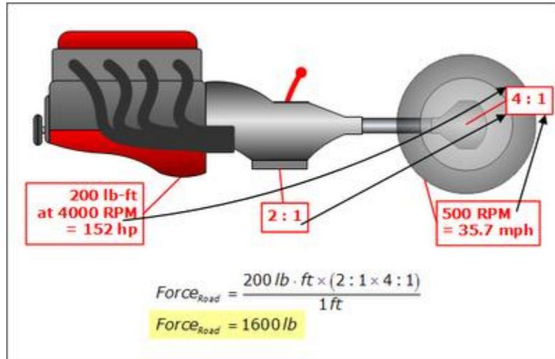
*The red engine makes 152 horsepower, which is twice the power of the other two engines. It is putting a 1600 lb force to the road, which is also twice as high as the other two engines.*
