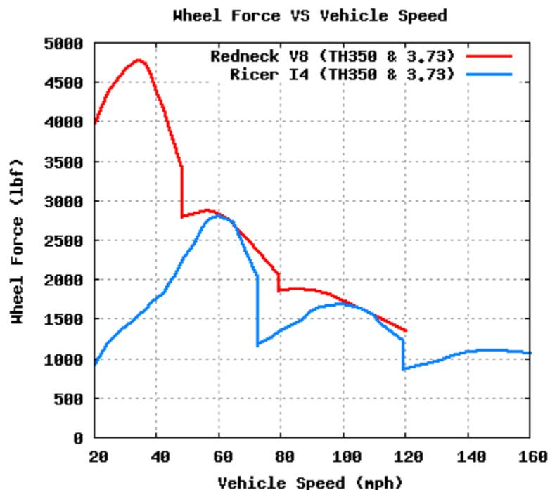
*Figure 4: Plot of rear wheel force versus vehicle speed for Redneck and Ricer when using a TH350 transmission and 3.73 axle ratio. The steep vertical drops are the gear changes at redline. Gear changes take place instantaneously for simplification.*
