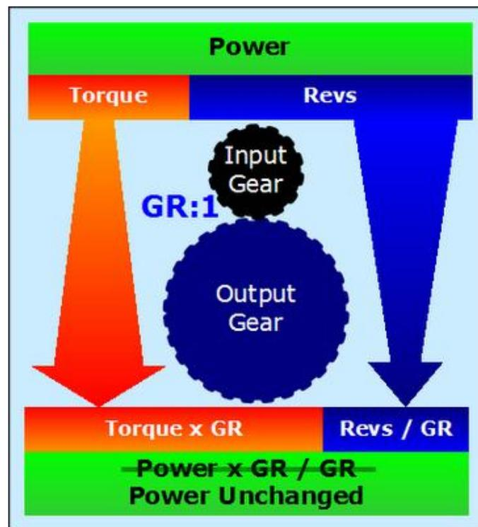
*The gearbox is given a certain amount of power, in the form of torque and revs. It then puts out an equal amount of power, with the revs and torque adjusted according to the gear ratio.*
