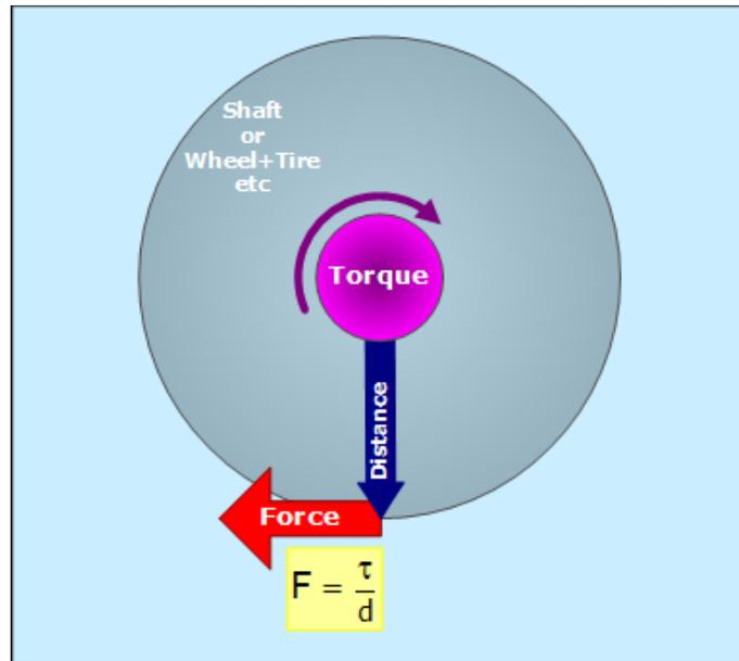
*Torque can be used to create a force at a distance, as seen below.
