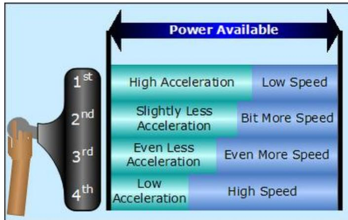
Each transmission gear provides a different amount of acceleration and speed. The combination of speed and acceleration is related to the power from the engine.
