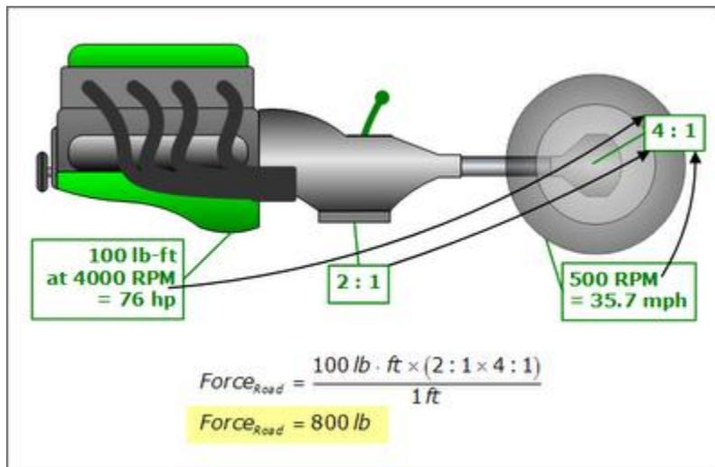
The green engine makes 76 hp and puts down 800 lbf to the road just like the blue engine.
