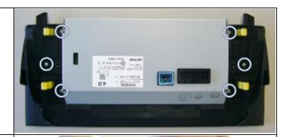
Remove the rear cover by pulling slightly upwards at the pins.
