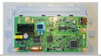
If available, we advice the rework to be performed on the desktop anti static mat used in the hybrid overhaul (SST: 09890-47010)
