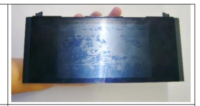
Slightly tilt away the front cover from the multi-display's LCD panel.
