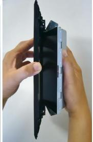
Remove the front cover and hold the LCD panel in you hand.
