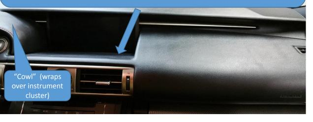
3) This leaves the entire silver trim piece exposed. It snaps out – remove RH end first. Be careful not to break the piece – it's thin in the center area behind the display. Photo show RH end loose.
