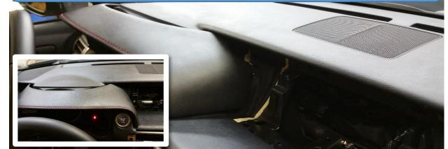
Removing LH end requires twisting piece around a bit, even with cowl loosened. This bent/broke a tiny pre-guide finger on the part, which is inconsequential – presumably it is an assembly aid/locating finger.
