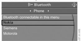
Select the desired mobile phone and press the controller
