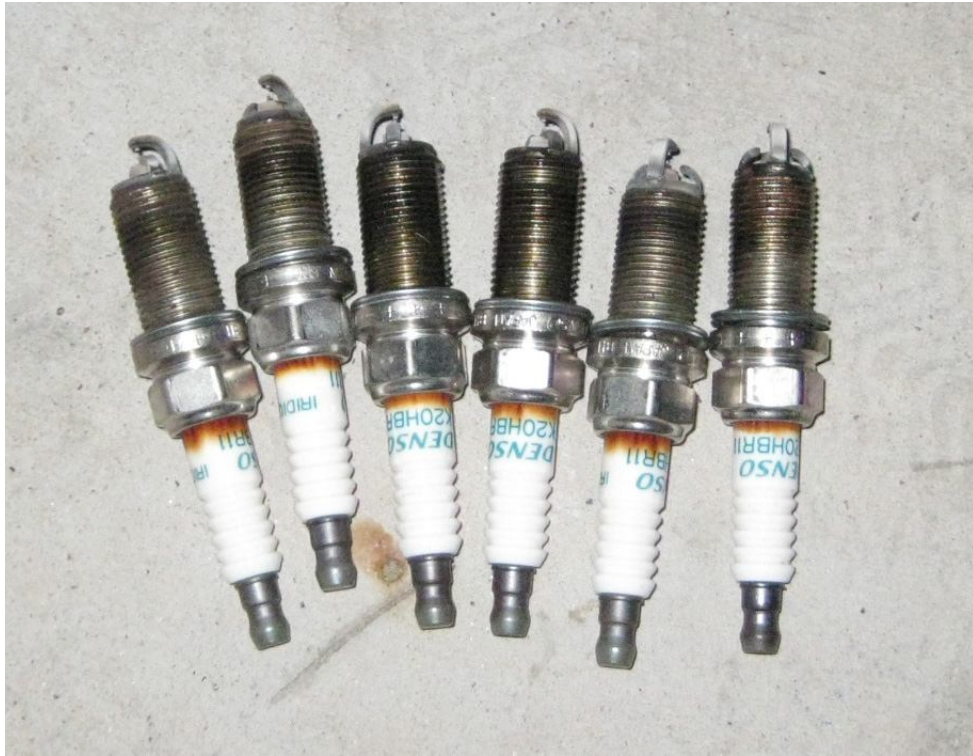
Figure 13 - These are my old plugs. Is it worth it to change them in 60000 mile interval? You decide.
