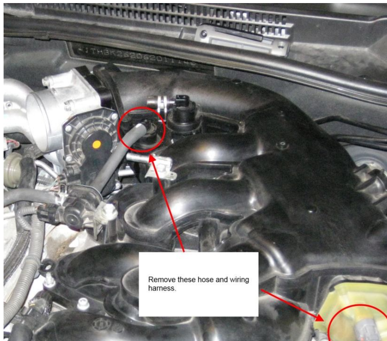
Figure 6 - Remove the vacuum hose and a wiring harness.
