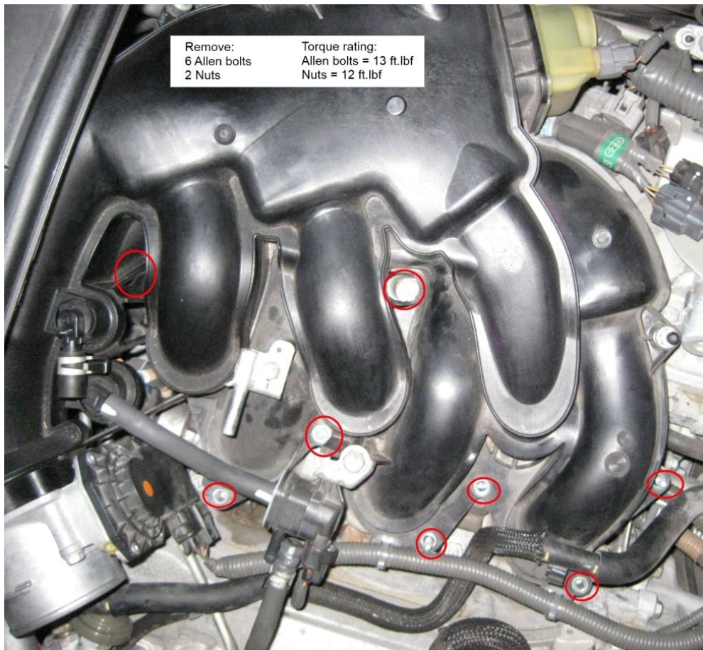
Figure 7 - The location of the Allen bolts and nuts. Use 10mm socket and 5mm Allen key.
