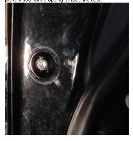
Remove the white electrical connector in the round hole that goes to the latch mechanism.
