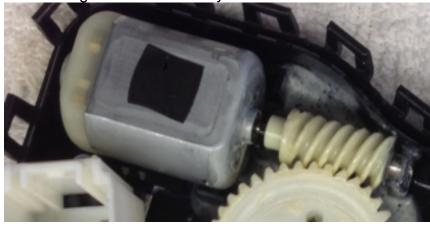
10mm Flat Shaft, FC-280PC-22125 Door Lock Motor Fix Repair Actuator Toyota Lexus is the one to buy if you need "D" shaft (I used on my 2008 for all 4 doors). \$6.50 from zinky86 on ebay.
