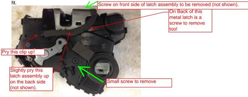
There is also a steel fork in the latch that engages a ~4 mm diameter white plastic shaft.
