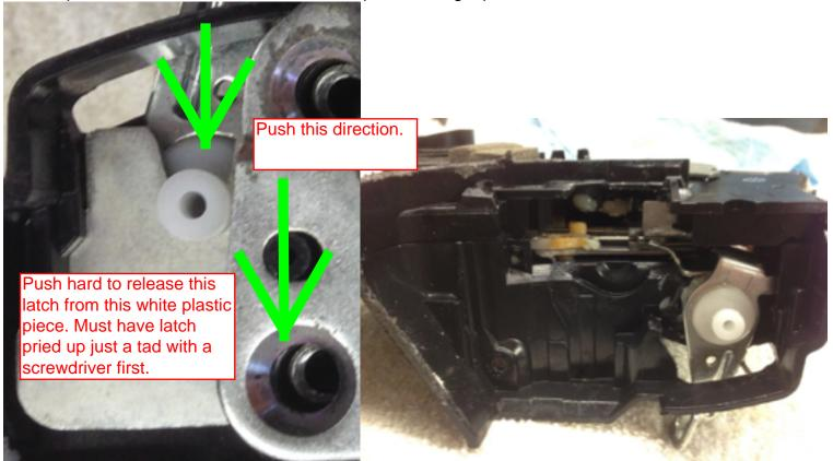
After you start the steel latch upwards in the slots, pry the steel fork off the white plastic shaft. You can use pliers gently if needed. After the shaft unsnaps, the latch will slide up and out of the main grooves.
