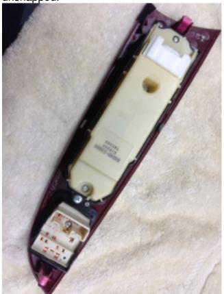
Disconnect the two white electrical connectors at the window and lock switches.
