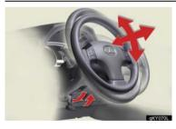
To adjust the steering wheel, press the lever down and move the steering wheel to the desired position. Lock the steering wheel in place by pulling the lever up.
