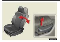
With the lever raised, tilt the seatback forward or backward.
