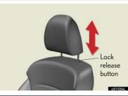
To raise: pull the head restraint upward. To lower: push the head restraint down while pressing the lock release button.
