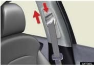
To raise: pull the anchor upward. To lower: depress the button and push the anchor down.
