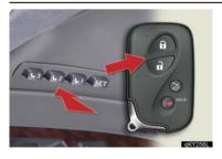
While holding down the desired memory button, press and hold either the **a** or **a** button on the wireless remote control until you hear a beep.
