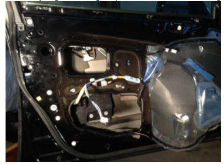
Remove the three Torx screws on the door rear face (jamb) holding the latch mechanism. Hold the latch from inside as you remove the last one.
