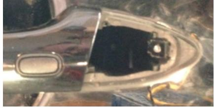
Removing the key socket makes removing the latch mechanism easier, and the key socket is easy to remove and install. When its time to reinstall the latch mechanism, having the key socket out is extremely helpful, maybe even required.
