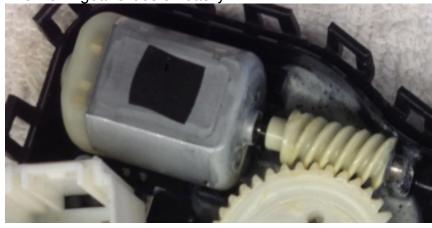
The Lexus motor has a "D" shaft and the eBay motor does not. A Dremel or file can remedy this difference.
