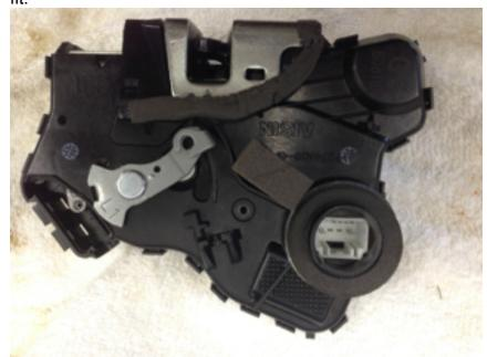
There is also a steel fork in the latch that engages a ~4 mm diameter white plastic shaft.
