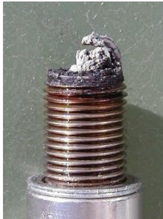
Figure 4 - An example of bad plug. Further diagnosis is needed if you encounter this. Taken from http://www.aa1car.com/library/fouled_sparkplug.jpg
