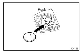
(e) Install a battery (lithium battery).
