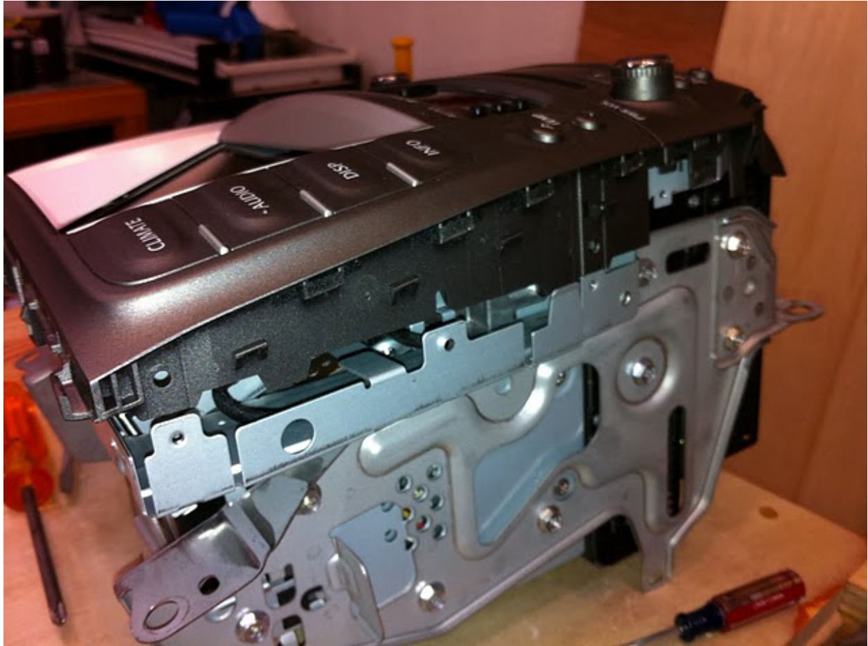
The navigation / stereo unit removed from dash. Four screws on this side have already been removed and the front panel has been lifted upwards for removal
