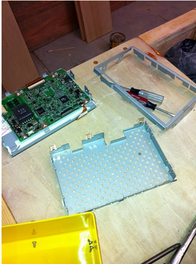
Here's the display, out and apart. Note the 4-wire ribbon connector going to the control board - that needs disconnected too and is the connector you make all the resistance measurements from
