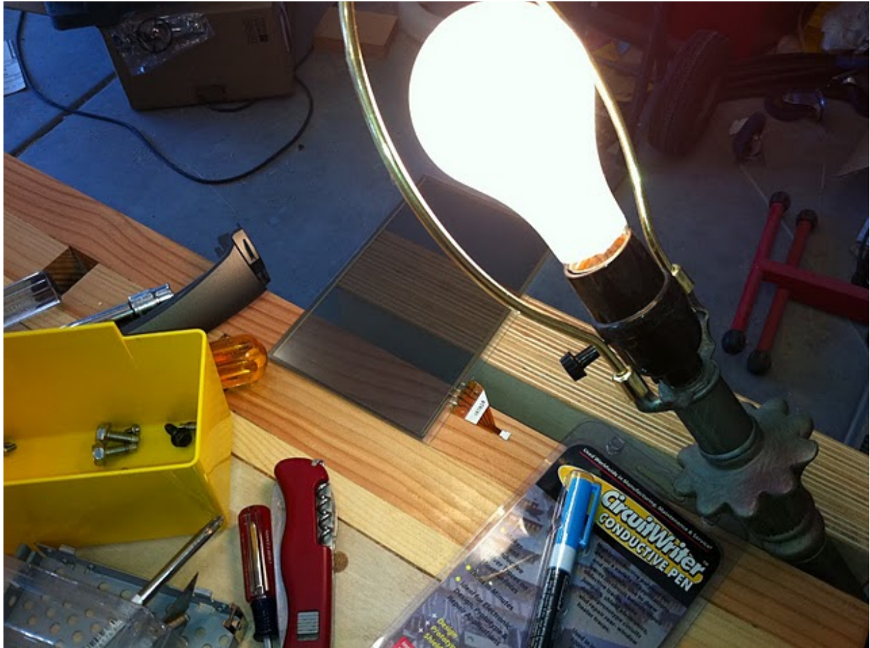
CircuitWriter pen + touch panel with repair "curing" under light. It doesn't conduct until dry
