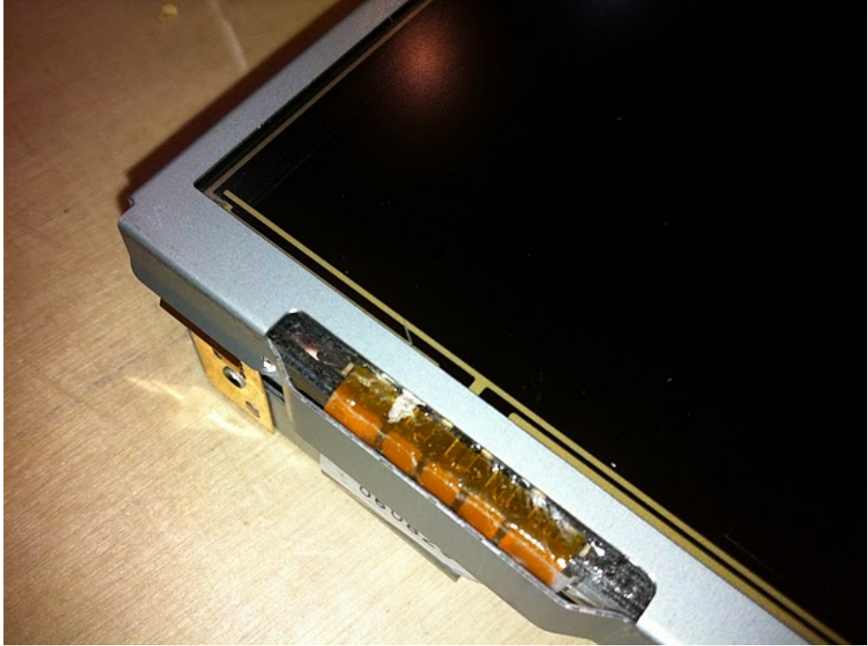
Panel reassembled, repaired trace visible
