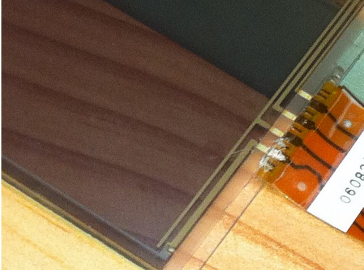
Connection repaired with Circuit tracer pen after using razor to expose copper on trace, and whittle away a bit of the edge of the glass.
