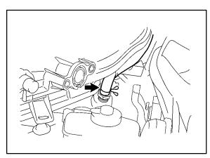
G. Connect the wire harness and hose to the intake air surge tank.
