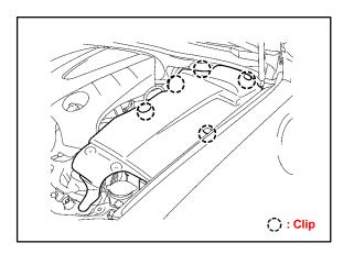
4. Remove the engine compartment side cover RH by removing the 2 clips.
