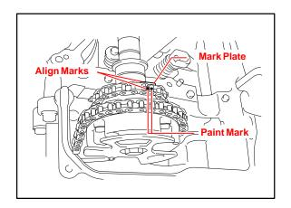
D. Hold the No. 2 chain and install the No. 3 chain tensioner assembly.
