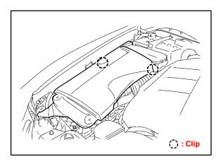
72. Install the cool air intake duct seal with the 11 clips.
