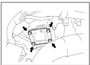
44. Install the injector driver with the bolt and 2 nuts.
