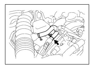
62. Install the No. 1 air cleaner inlet with the 2 bolts.
