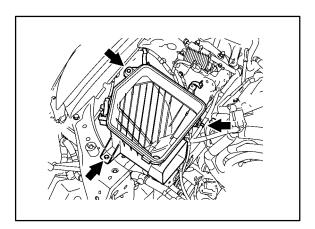
11. Disconnect the union to check valve hose by removing the clamp.
