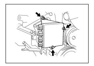
45. Install the No. 1 engine cover with the 3 clips.
