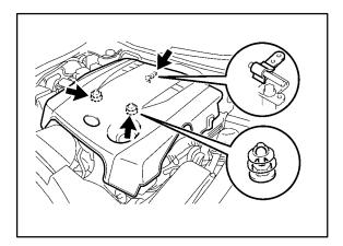
70. Install the engine compartment side cover LH with the 5 clips.
