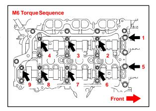
E. Tighten the 9 M8 bolts in the sequence shown in the illustration.
