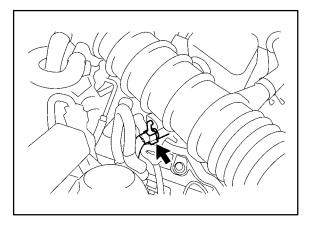
C. Connect the MAF connector and clamp to the air cleaner.
