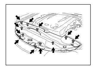
3. Remove the engine compartment side cover LH by removing the 5 clips.
