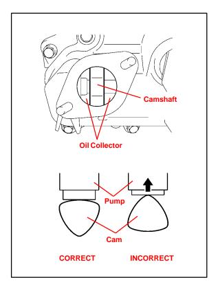
C. Apply a coat of engine oil to the pump activation cam and pump lifter part.
