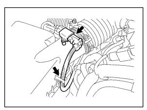
61. Connect the No. 2 ventilation hose to the cylinder head cover with the clamp.
