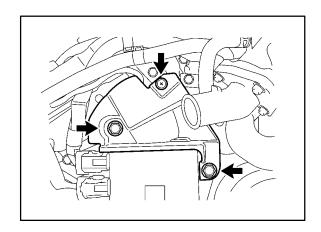
25. Remove the injector driver by removing the bolt and 2 nuts.
