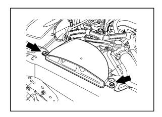
8. Disconnect the No. 2 ventilation hose from the cylinder head.
