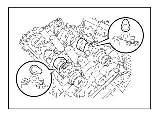
B. Uniformly loosen and remove the 9 camshaft bearing cap M6 bolts in the sequence shown in the illustration.
