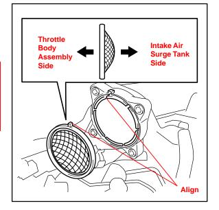
B. Install the throttle body with the 4 bolts.
