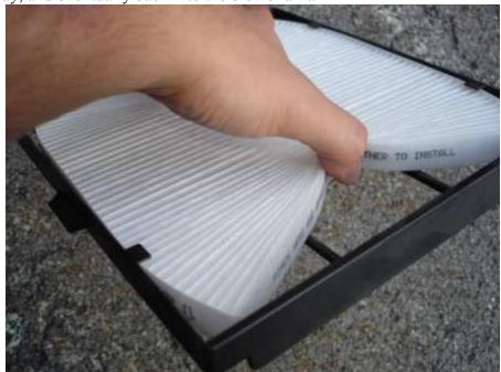
To better understand what I mean, think a few steps ahead to when you reinstall the tray into the blower unit and picture the blower sucking air through the filter into the HVAC unit. This is the direction you want the arrow to be pointing when you install the new filter. Let's look at a picture of the old filter. The arrows show the direction of flow of the air, from outside to inside into the HVAC unit. You can tell by the dirt also, which way the air flows:
