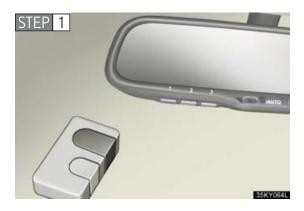
Point the remote control for the device 1 to 3 in. (25 to 75 mm) from the  $HomeLink^{\circledR}$  control buttons.
