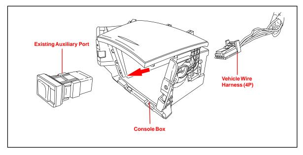
Repair Procedure (Continued) Install the revised auxiliary port, wire harness, and noise filter.
