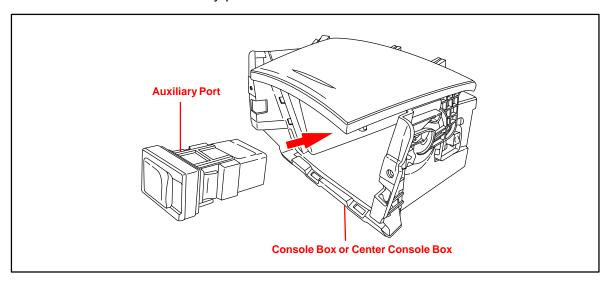
D. Connect the filter wire connector (8P) into the NEW auxiliary port.
