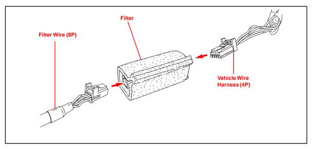
B. Secure the filter to the vehicle wire harness using wire ties.
