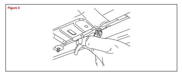
4. Reassemble the headliner in reverse order. For proper installation procedures, refer to TIS, 2006 model year GS 300 or GS 430 Repair Manual: Interior: *Headlining: Installation.*
