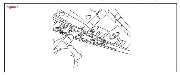
3. Cut off the tip of the back window glass stopper, located at each upper corner of the rear glass. (Refer to Figures 2 and 3.)
