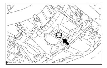
a. Loosen the bleeder plug shown in the illustration and connect a hose.
