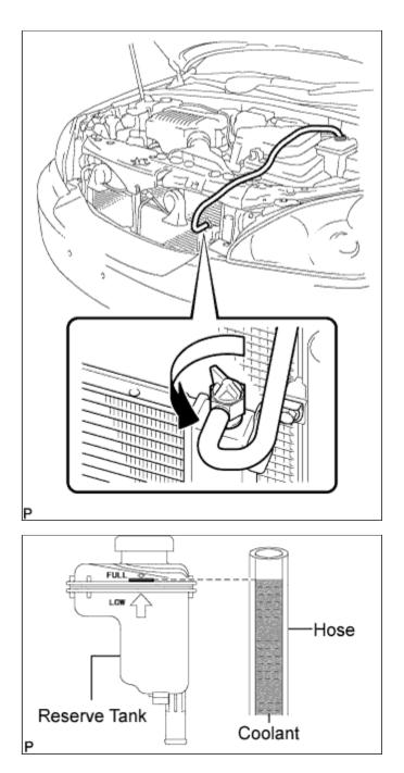
**c.** Add coolant until the level of coolant in the hose attached to the bleeder plug reaches the same level as the FULL line of the reserve tank.
