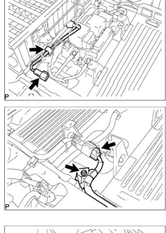
ii. Remove the nut, then disconnect the main battery cable connector.
