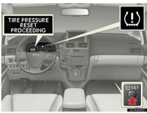
STEP 5 Wait for a few minutes with the "POWER" switch in ON mode and then turn the "POWER" switch off.
