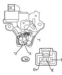
(b) Move the door lock to the closed (locked) position.
