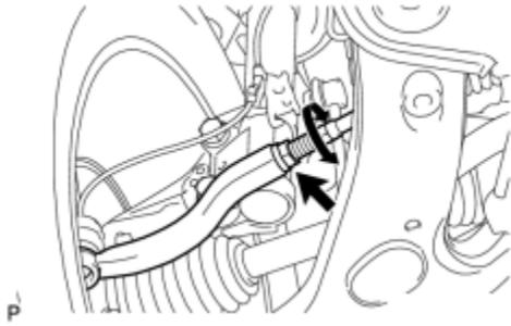
(d) Adjust the rack ends if the difference in thread length between the right and left rack ends is not within the specified range.
