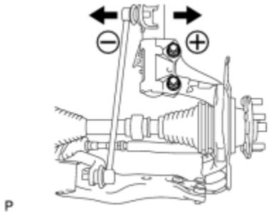
(e) Fully push or pull the front axle hub in the direction of the required adjustment. (Step B)
