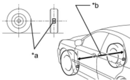
(d) Put tread center marks on the rearmost points of the front wheels and measure the distance between the marks (dimension B).
