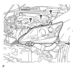
(a) Remove the bolt and 3 screws.
