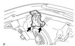
(b) Install the upper headlight protector retainer with the 2 screws.
