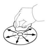
(1) If dirt is on the disc surface, wipe it clean with a soft dry cloth such as an eyeglass cleaner for plastic lenses from the inside to the outside in a radial direction.
