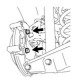
(a) Remove the 2 bolts and rear disc brake cylinder mounting from the rear axle carrier sub-assembly.
