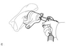
(a) Place a piece of cloth between the rear disc brake piston and rear disc brake cylinder assembly.
