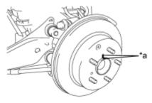
(a) Put matchmarks on the rear disc and the axle hub.
