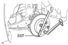
(b) Using SST to hold the rear disc, tighten the rear disc with the 5 hub nuts.
