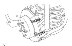
(a) Remove the 2 rear disc brake pad support plates from the disc brake cylinder mounting.
