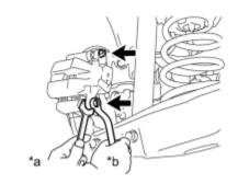
(a) Hold the 2 rear disc brake cylinder slide pins and install the rear disc brake cylinder assembly to the rear disc brake cylinder mounting with the 2 bolts.
