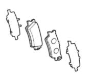
(a) Install the rear disc brake anti-squeal shims to each of the 2 rear disc brake pads.
