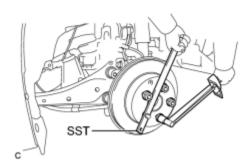
(b) Using SST to hold the rear disc, tighten the rear disc with the 5 hub nuts.
