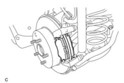
(a) Install the 2 rear disc brake pads to the rear disc brake cylinder mounting.
