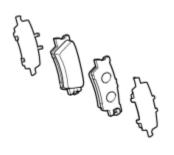
(a) Remove the 2 rear disc brake anti-squeal shims from the rear disc brake pads.
