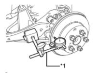
(c) Using a dial indicator, measure the disc runout 10 mm (0.394 in.) away from the outer edge of the rear disc.
