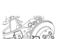
(c) Using a dial indicator, measure the disc runout 10 mm (0.394 in.) away from the outer edge of the rear disc.
