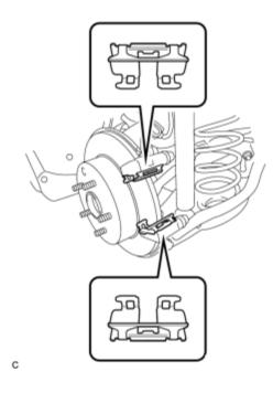
(a) Install the 2 rear disc brake pad support plates to the rear disc brake cylinder mounting.
