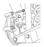
(e) Install the rear disc brake cylinder slide pin (upper) to the rear disc brake cylinder mounting.
