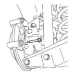
(b) Remove the rear disc brake cylinder slide pin (lower) from the rear disc brake cylinder mounting.
