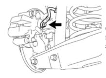
(a) Remove the union bolt and gasket, and disconnect the rear flexible hose from the rear disc brake cylinder assembly.
