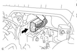
(a) Connect the connector to the brake booster with master cylinder assembly.
