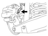
(a) Connect the rear flexible hose to the rear disc brake cylinder assembly with a new union bolt and a new gasket.
