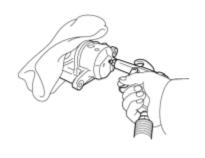
(a) Place a piece of cloth between the front disc brake piston and disc brake cylinder assembly.
