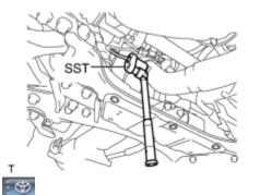
(b) Using SST, remove the oxygen sensor from the front exhaust pipe assembly.
