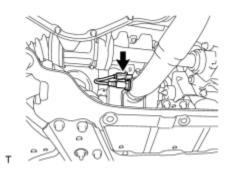
(a) Disconnect the oxygen sensor connector.
