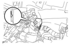
(b) Engage the claw to install the turn signal flasher assembly.
