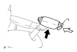
(c) Gradually attach the rain sensor to the glass surface to prevent air bubbles from forming between them.
