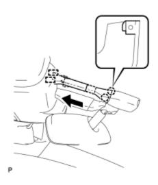
(a) Engage the 2 claws and connect the rain sensor cover.
