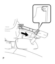
(a) Disengage the 2 guides and disconnect the rain sensor cover as shown in the illustration.
