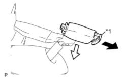
(b) Release the stopper by pulling the stopper down and disconnect the rain sensor as shown in the illustration.
