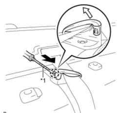
(b) Using a screwdriver with the tip taped, disengage the claw to open the cap of the rear seat center shoulder belt guide.
