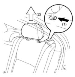
(a) Press the headrest support button and pull up the rear seat headrest assembly LH as shown in the illustration.
