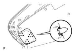
(a) Disengage the 3 clips and remove the luggage compartment trim cover assembly LH.
