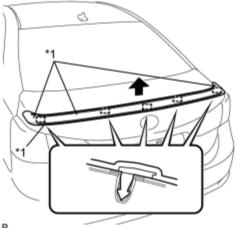
(b) Disengage the 5 pins to remove the rear upper spoiler sub-assembly.
