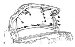
(a) Disengage the 12 clips and remove the luggage compartment door cover.
